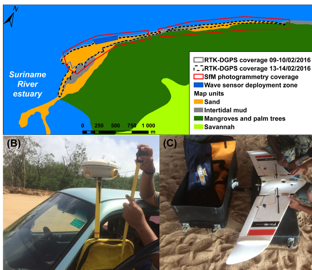
FIGURE 3 | (A) Experiments conducted on Braamspunt beach in February, 2016 and their ground coverage; (B) mobile GPS station on an all-terrain vehicle; (C) drone with custom-built wings used for photogrammetric survey.
